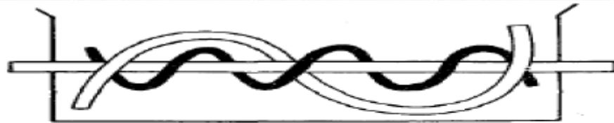
FIG. 1-12. Side view of a top-loading ribbon blender. The blades are mounted on the horizontal axle by struts (not shown) and are rotated to circulate the material to be mixed. The spiral blades are wound (in most cases) in opposite directions to provide for movement of material in both directions along the axis of the tank. These mixers may be emptied either through ports in the bottom or by inverting them.
