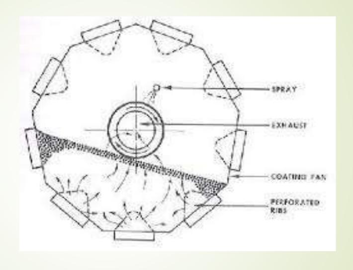
In the Glatt coater, drying air can be directed from inside the drum through the tablet bed and out an exhaust duct.
