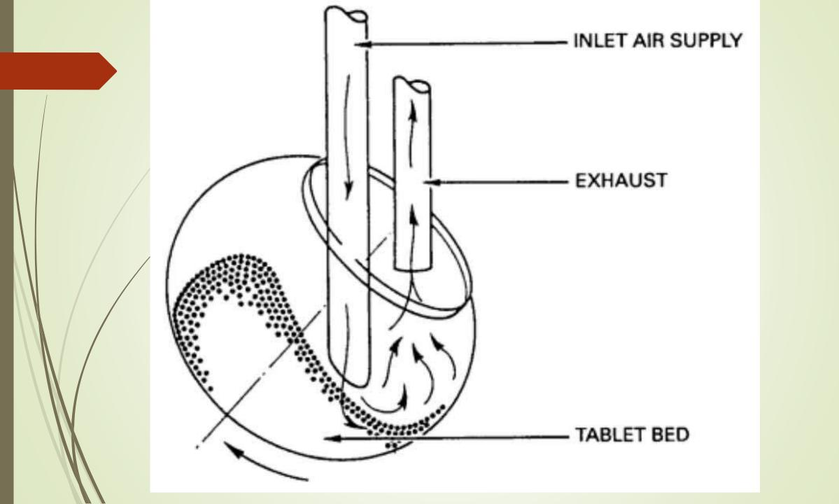
Coating solutions are applied to the tablets by ladling or spraying the material onto the rotating tablet bed. Use of atomizing systems to spray the liquid coating material onto the tablets produces a faster, more even distribution of the solution or suspension.
