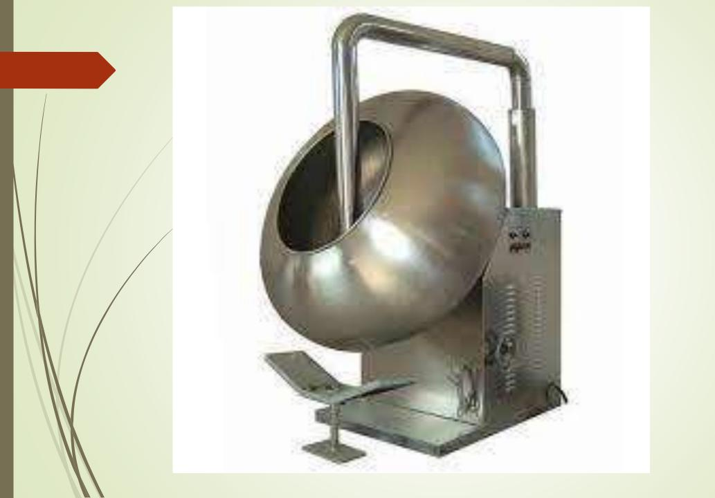
Heated air is directed into the pan and onto the tablet bed surface, and is exhausted by means of ducts positioned through the front of the pan.
