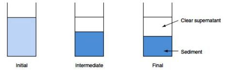
. The sedimentation behaviour of a flocculated suspension. Pale blue colouration indicates the initial
