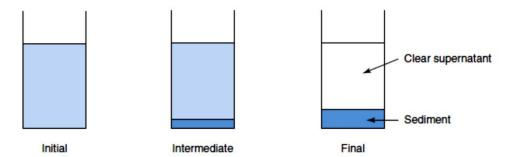
The sedimentation behaviour of a deflocculated suspension. Pale blue colouration indicates th
