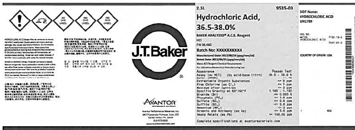
Figure 4-1 Label from a bottle of reagent-grade hydrochloric acid. Note that the specific gravity of the acid over the temperature range of 60° to 80°F is specified on the label. (Label provided by Mallinckrodt Baker, Inc., Phillipsburg, NJ 08865)
